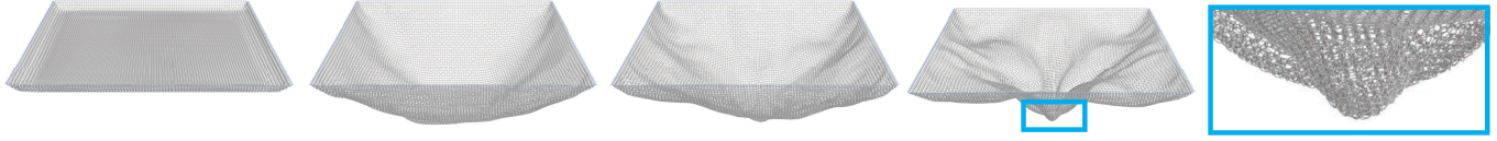
Fig. 15. Huge chain net. When the body count increases, the disadvantage of using redundant DOFs in the simulation may become more obvious. Following this thought, we up scale the chain net to 27,645 bodies. In this stress test, A-IPC takes about 5 min to simulate one frame on average. The entire simulation takes about five days with A-IPC. We are never able to finish this test with rigid-IPC. Based on our observation, A-IPC is at least 2,000× faster than rigid-IPC. This means it will need several years for rigid-IPC to finish this experiment.
