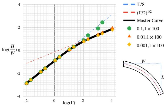
**Figure 7: Comparison with theoretical solutions. We superimpose our results of the 2D cantilever beam simulation onto the master curve presented in Romero et al. [2021]. The blue and red dashed lines correspond to the asymptotic expressions for small and large  $\Gamma$ . Our results quickly converge to the master curve as the thickness of the beam decreases.**
