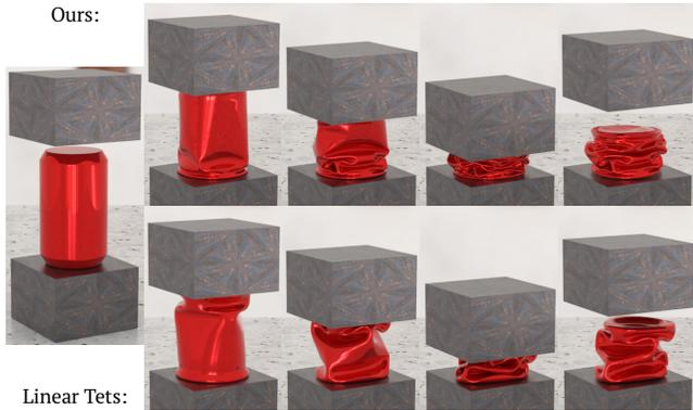
**Figure 10: Coke can.** Using real-world aluminium parameters, our method (top) can generate sharp wrinkles and buckling on the compressed coke can, while Li et al. [2022] (bottom) suffers from severe shear locking issues.
