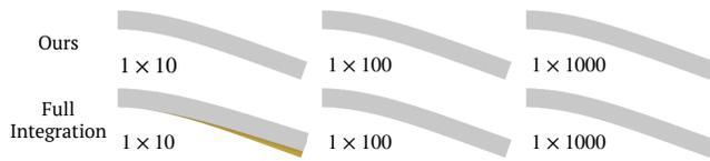
**Figure 6: 2D cantilever beam. Static equilibrium of a 2D cantilever beam (left end fixed) under gravity simulated using our element with different integration schemes, where higher full integration is adopted as the reference. Our results converge early even with a single layer of 10 elements, while full integration converges slower.**
