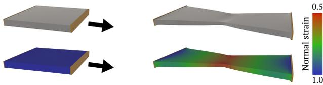
**Figure 9: Metal board.** Elongating a metal board, the smooth thickness decreases and plastic deformations are effectively captured by our method.
